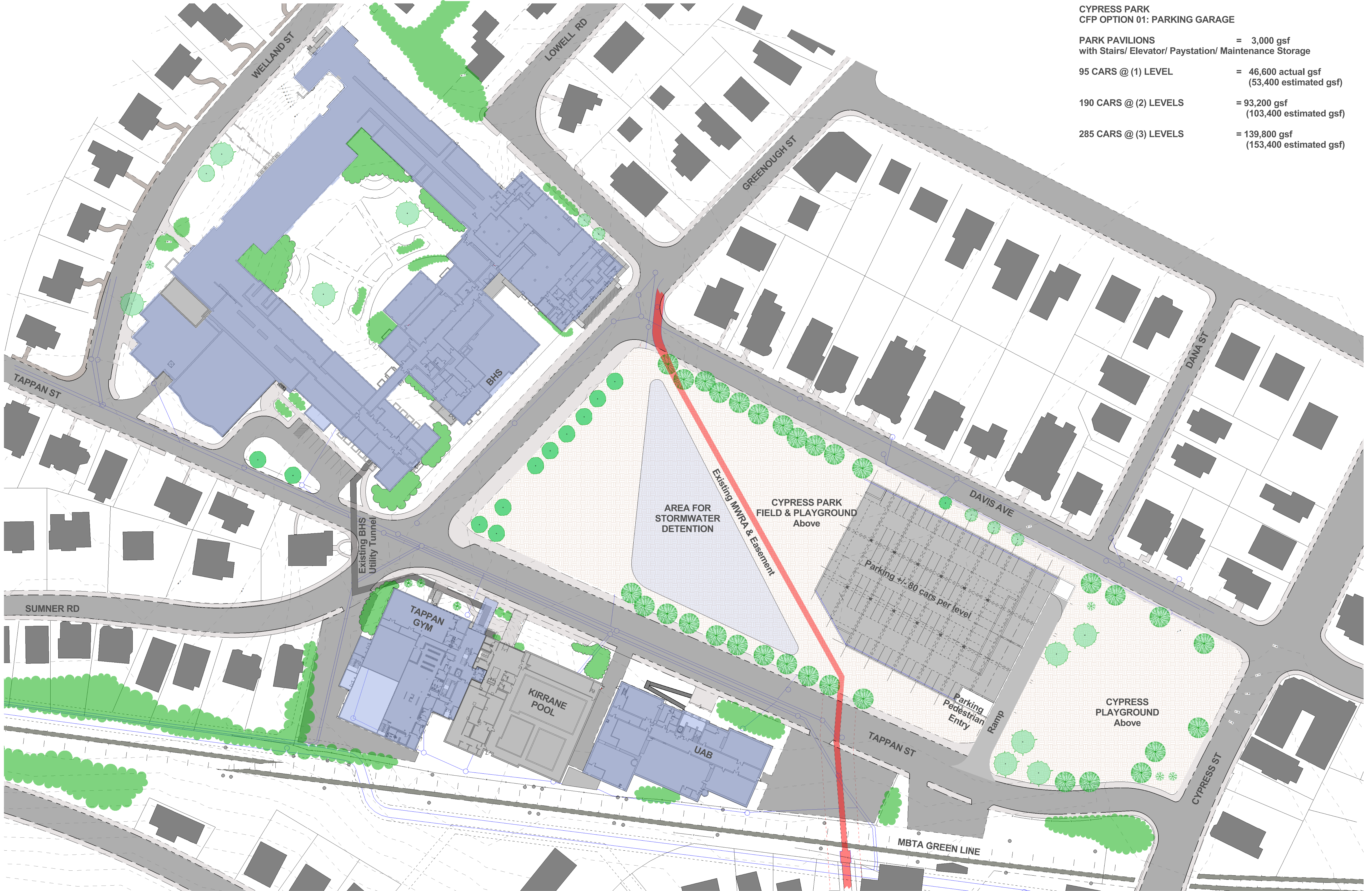
Cypress Park Site Plan - Below Grade Parking Brookline High School Brookline, MA 09 March 2017
